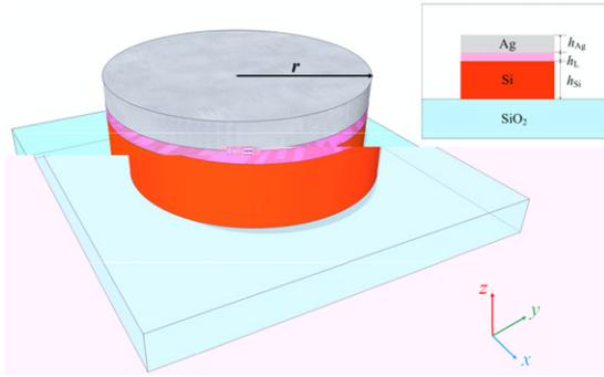
**Figure 1.** Schematic diagram of the HP nanodisk. The inset shows the cross-section of the HP nanodisk: the silicon layer has a height  $h_{Si}$ ; the low-index layer has a height  $h_L$ ; and the silver layer has a height  $h_{Ag}$ .
