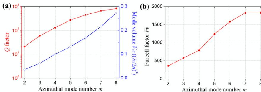
**Figure 3.** (a) The dependence of the  $Q$  factor (solid) and the mode volume (hollow) on the azimuthal mode number  $m$ . (b) The dependence of the Purcell factor on the azimuthal mode number  $m$ .
