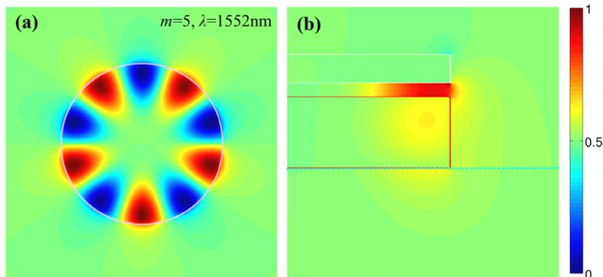
**Figure 2.** (a) The  $E_z$  field distribution in the center of the low-index layer for an HP nanodisk with the radius  $r = 670$  nm at  $\lambda = 1552$  nm ( $m = 5$ ). The solid line shows the edge of the low-index layer. (b) The  $E_z$  field distribution in the  $x$ - $z$  plane (half). The solid lines show the silver and silicon layer and the dashed line shows the surface of the silica layer.
