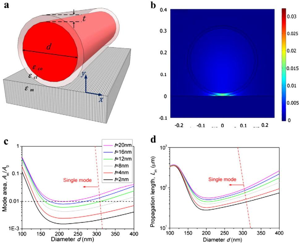
**Fig. 1.** (a) Schematic picture of the HP waveguide. A high index dielectric core (diameter  $d$ ) with a low index cladding (thickness  $t$ ) sits on a metallic substrate. (b) Electromagnetic energy density distribution for the HP waveguide with diameter  $d = 200$  nm, thickness  $t = 10$  nm (c) Normalized mode area  $A_m/A_0$  and (d) propagation length  $L_m$  versus the diameters  $d$  and thicknesses  $t$ .
