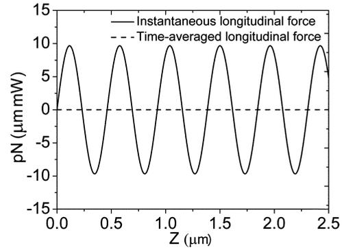
FIG. 1. The solid line shows the instantaneous longitudinal force distribution as a function of  $z$  for a typical SD silica fiber with a diameter of 450 nm and incident light with a wavelength of 980 nm. The dashed line shows the time-averaged longitudinal force.
