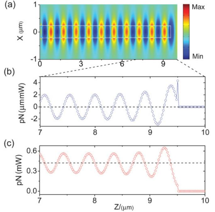
FIG. 3. (Color online) (a) Computed instantaneous  $E_x$  distribution on the  $x$ - $z$  ( $y = 0$ ) cross-sectional plane. The white line represents the profile of the fiber. (b) Time-averaged Lorentz force over the transverse cross-sectional plane  $F_z$  as a function of  $z$ . (c) Integrated  $F_z$  from the fiber end face to a position where  $z < 9.5 \mu\text{m}$ .
