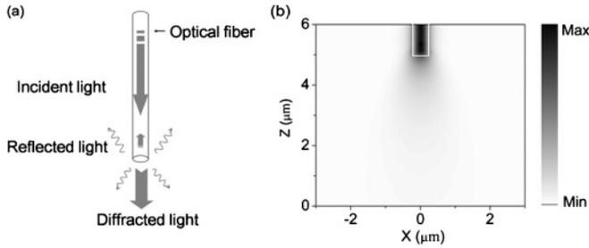
FIG. 2. (a) Schematic of the reflected and diffracted light at the end face of the SD fiber. (b) Calculated  $z$ -direction Poynting vector distribution in the  $x$ - $z$  ( $y = 0$ ) cross-sectional plane for a 450-nm-diam silica fiber with a refractive index of 1.45 at a wavelength of 980 nm (quasi- $x$ -polarized). The white line represents the profile of the fiber.
