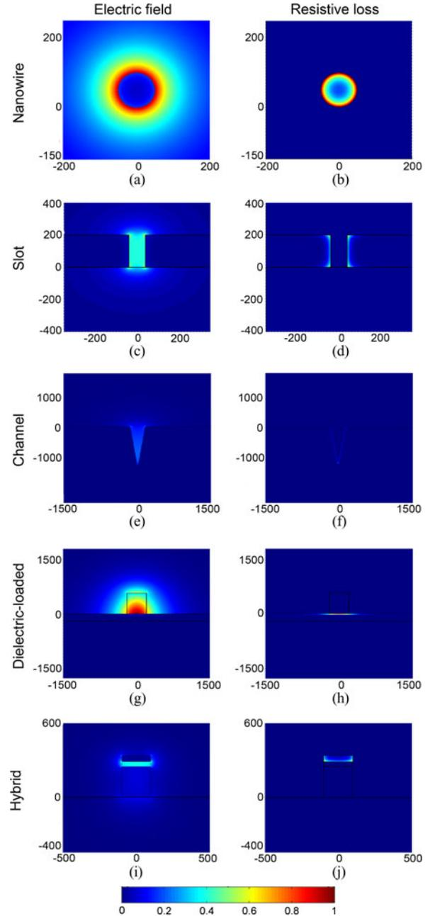
Fig. 2. Normalized electric field and resistive loss for the five Au PWs. (a) and (b) Nanowire PW with  $r = 50 \text{ nm}$ , (c) and (d) slot PW with  $W_2 = 80 \text{ nm}$  and  $H_2 = 200 \text{ nm}$ , (e) and (f) channel PW with  $W_3 = 320 \text{ nm}$  and  $H_3 = 1200 \text{ nm}$ , (g) and (h) dielectric-loaded PW with  $W_4 = 400 \text{ nm}$  and  $H_4 = 600 \text{ nm}$ , and (i) and (j) hybrid PW with  $W_5 = 200 \text{ nm}$  and  $H_5 = 250 \text{ nm}$ .
