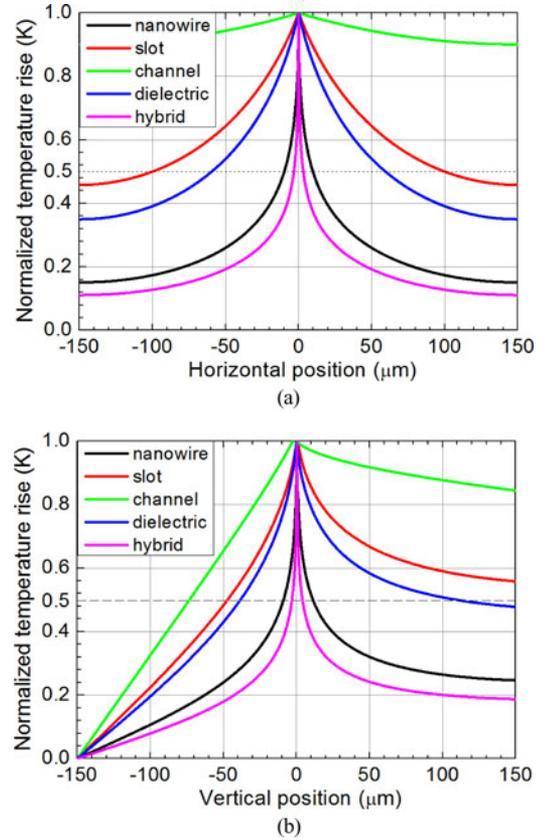
Fig. 4. Spatial distribution of temperature rise in (a) the horizontal ( $x$ -direction) and (b) vertical direction ( $y$ -direction) for the five Au PWs. The temperature rises are normalized to the maxima. The geometrical parameters are the same as those shown in Fig. 2.
