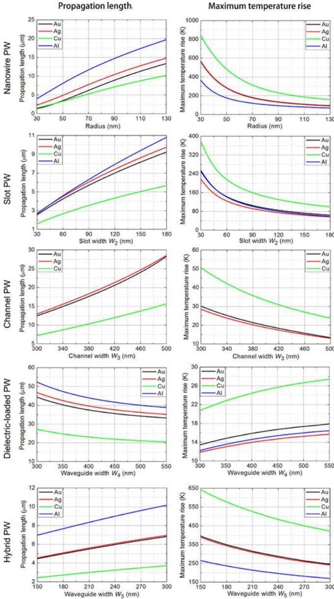
Fig. 5. Dependence of (left) effective propagation length and (right) maximum temperature rise on nanowire radius/waveguide width. The geometrical parameters are the same as those shown in Fig. 2 except the nanowire radius/waveguide width.
