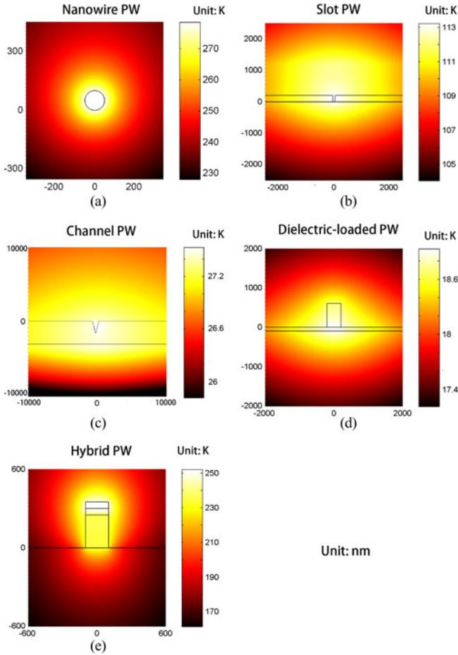
Fig. 3. Temperature rise profiles for the five Au PWs. The geometrical parameters are the same as those shown in Fig. 2.
