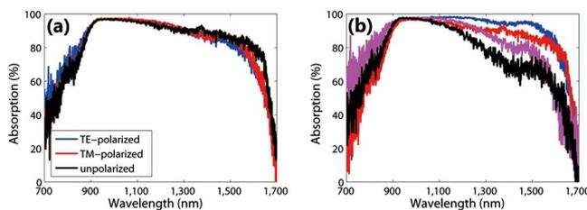
Fig. 2. (a) Absorption spectra for different polarizations of the light: unpolarized (black curve), TE-polarized (blue curve), and TM-polarized (red curve) light. (b) Absorption spectra at different randomly chosen locations of the metasurface.
