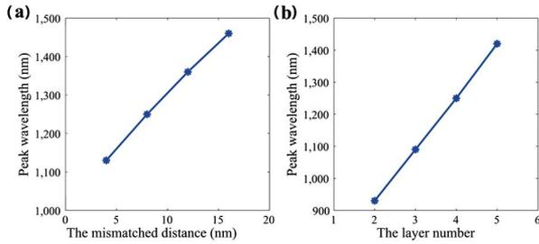
Fig. 4. Peak wavelength versus the mismatched distance and layer number. Peak absorption wavelength (a) as a function of the mismatched distance  $d$  at  $N = 4$  and (b) as a function of the layer number  $N$  at  $d = 8$  nm.
