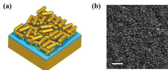
Fig. 1. Morphology of the nanostructure based on multilayer gold nanorods. (a) Schematic diagram of the metasurface consisting of three layers: gold nanorods randomly dispersed on a gold film spaced by a dielectric layer. (b) Scanning electron microscope image of the gold nanorods deposited on the dielectric surface. The scale bar is 200 nm.
