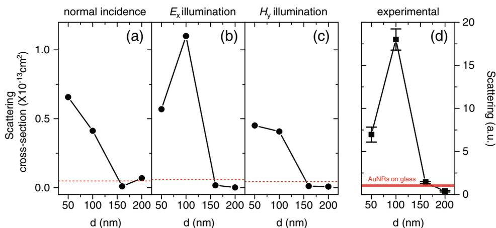
**Fig. 2** Magnitudes of scattering maxima for AuNRs at varied distances above a Au substrate under normal incidence (a),  $E_x$  (b) and  $H_y$  (c) illuminations. Dashed line in each panel indicates the scattering magnitude of AuNRs on a glass substrate under the same illumination conditions. **d** Experimentally acquired scattering magnitudes of AuNRs
