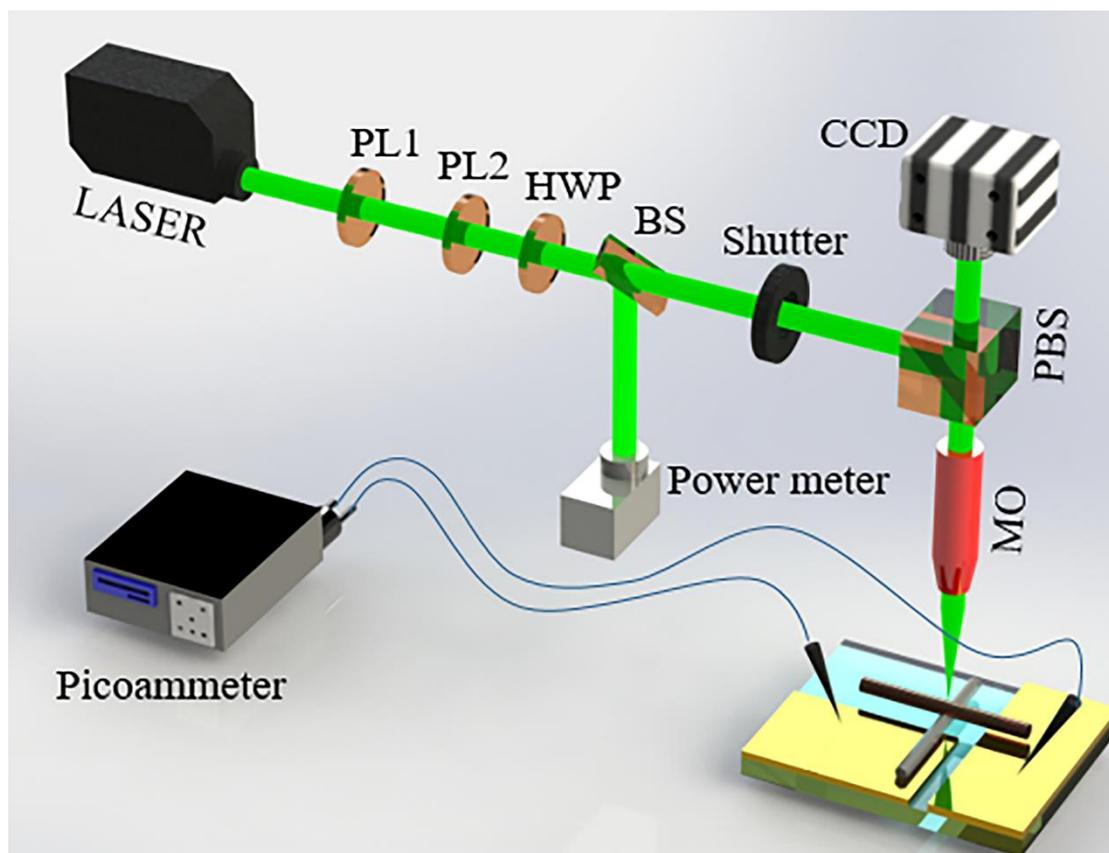
**Figure S1** Experimental setup for nanowelding and electrical characterization. PL1 and PL2 are the polarizers, HWP is the half wave plate, BS is the beam splitter, PBS is the Pellicle beam splitter, and MO is the microscope objective.
