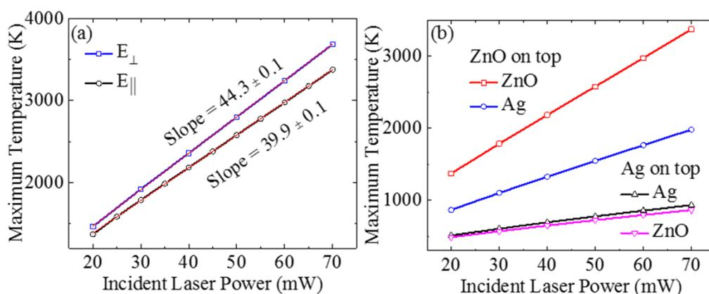
**Figure S2** Maximum temperature versus incident laser power plots for different incident laser beam polarization (a) and orientation (b) of the NWs. The diameter and length of the NWs are kept fixed at 300 nm and 10  $\mu\text{m}$ , respectively.
