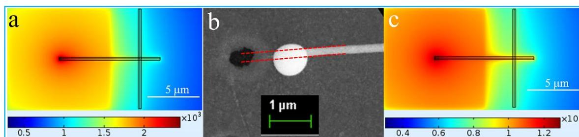
**Figure S4** (a) Simulated temperature distribution plots for welding ZnO NW on Au electrode corresponding to laser power 70 mW. (b) SEM images of welded Ag NW on Au electrodes. The dashed red lines represent the orientation of the NWs before welding. (c) Simulated temperature distribution plots for welding Ag NW on Au electrodes corresponding to laser power 60 mW.
