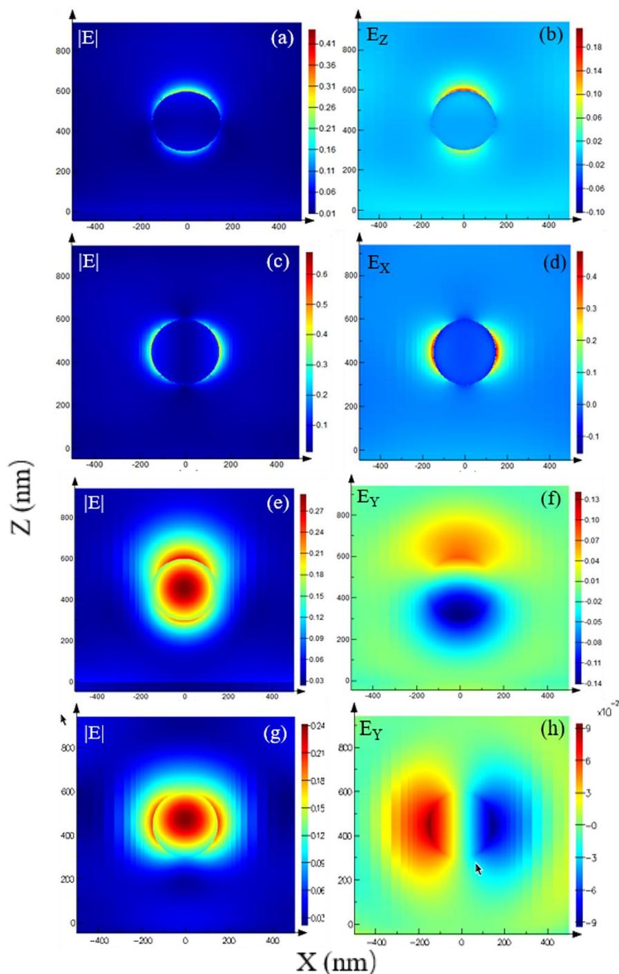
**Figure S5** Simulated electric field distribution corresponding to different orientation of the NWs and polarization of the incident laser beam. Electric field distribution at the end of Ag NW (a-d) and ZnO NW (e-h) when Ag and ZnO NWs are on top, respectively. (a, c, e, and g) Electric field magnitude. (b, d, f, and h) Dominant electric field component. (a, b, e, and f) Corresponding to parallel, and (c, d, g, and h) for perpendicular polarization of the incident laser beam.
