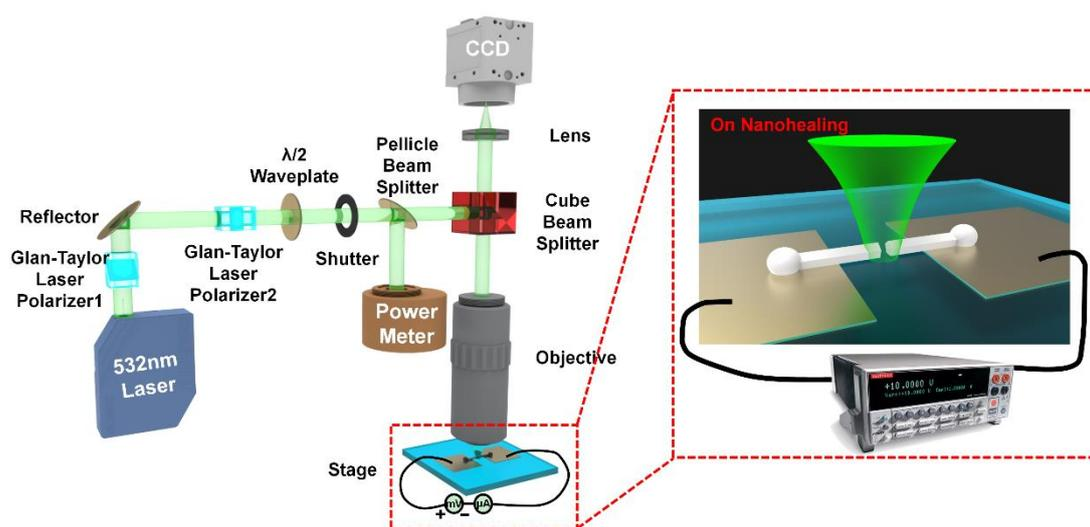
Figure S1. Schematic diagram of the experimental apparatus for nanoheating and electrical characterization
