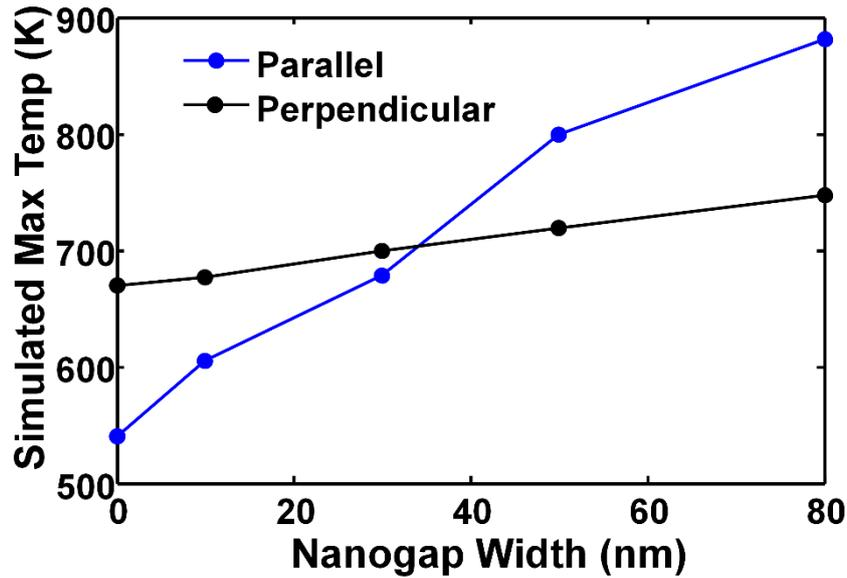
Figure S3. Simulated maximum temperature versus nanogap width under parallel and perpendicular polarization of the incident laser beam.
