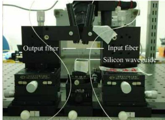
Fig. 6. Picture of the vertical coupling system.
