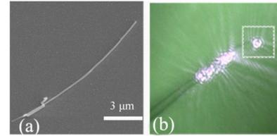
FIG. 3. (Color online) Hybrid plasmonic mode propagation in different waveguides. (a) SEM image of a 12.5  $\mu\text{m}$  long nanowire (170 nm in diameter). (b) Optical microscope image illustrating the experimental excitation of the plasmonic mode in the waveguide.
