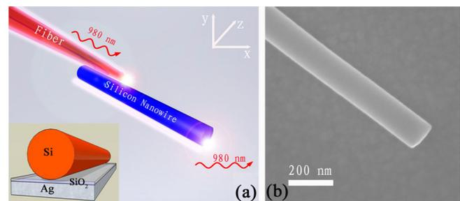
FIG. 1. (Color online) Nanoscale hybrid plasmonic waveguide. (a) The schematic of the plasmonic waveguide and its light in-coupling scheme. The inset is the cross section of the waveguide, showing the underlying layers. (b) The SEM image of a typical hybrid plasmonic waveguide.
