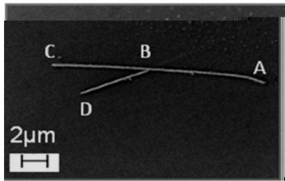
Fig. 7. SEM image of the nanosplitter.
