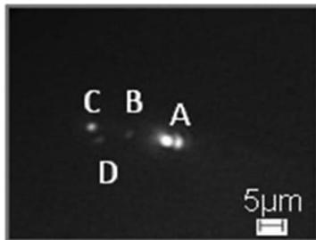
Fig. 8. Dark-field optical microscope image of the light propagation through the nanosplitter. Two bright light spots (C and D) are observed at the ends of the two branches of the nanosplitter.
