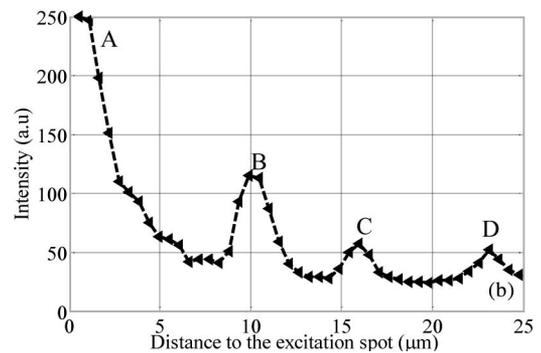
Fig. 6. (a) Optical microscope image illustrates the propagation of light along the nanowire coupler. (b) Intensity profile of the output light along the cut lines ABCD as indicated in (a).
