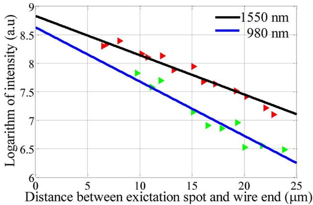
Fig. 4. Plot of the logarithm of output intensity from the end of the nanowire versus the distance the between excitation spot and the wire end. The black and blue solid lines represent fitting of the data to exponentially decaying functions at 1550 nm and 980 nm, respectively.
