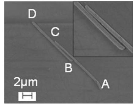
Fig. 5. SEM image of the nanocoupler. The inset shows a close-up image of the coupling region.
