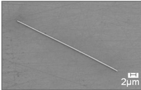
Fig. 1. (a) SEM image of a silver nanowire synthesized by a soft solution method. The nanowire has a diameter of 300 nm and a length of 45 μm.
