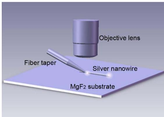
Fig. 2. Sketch of the optical excitation of SPP at 1550 nm in the silver nanowire.
